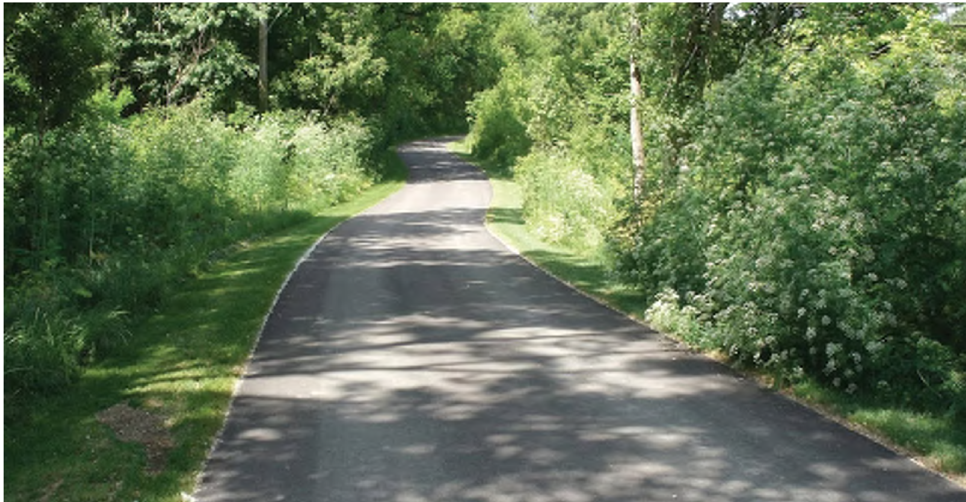
PRIMARY TRAIL (PAVED ASPHALT CONSTRUCTION (8' WIDE))
