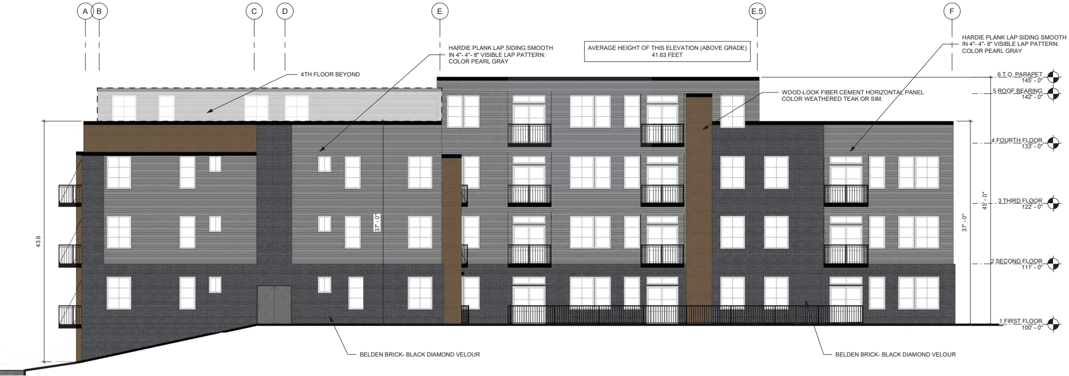
17 SOUTH EXTERIOR ELEVATION 1/8" = 1'-0"
