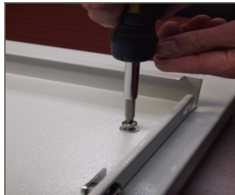
[Figure 4] Attaching the sign bracket.
