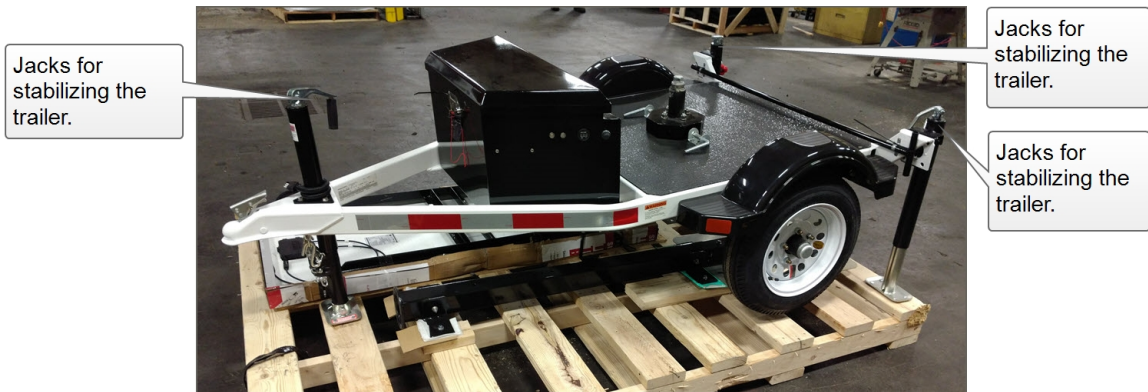
[Figure 27] Trailer with jacks deployed
