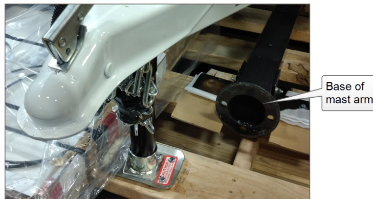
[Figure 1] Base of the mast arm
